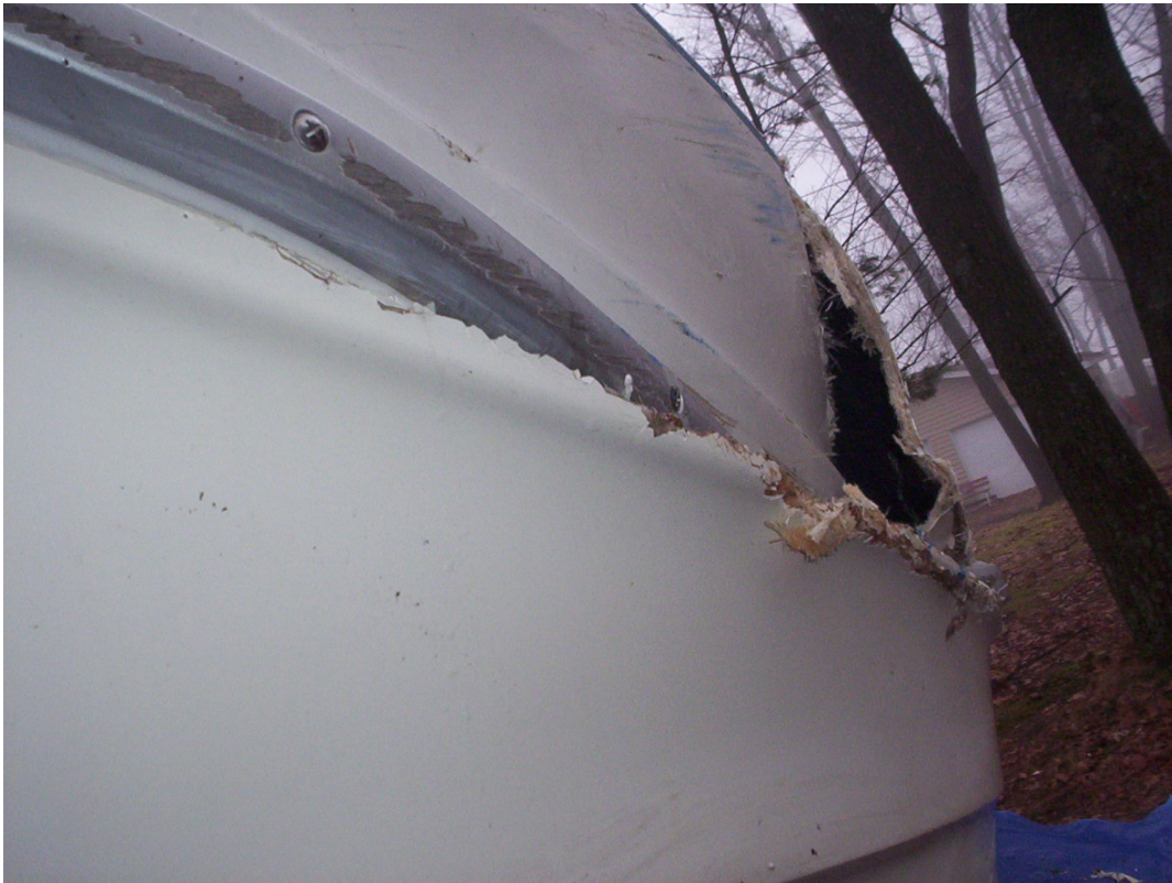
Deck and hull broken.
