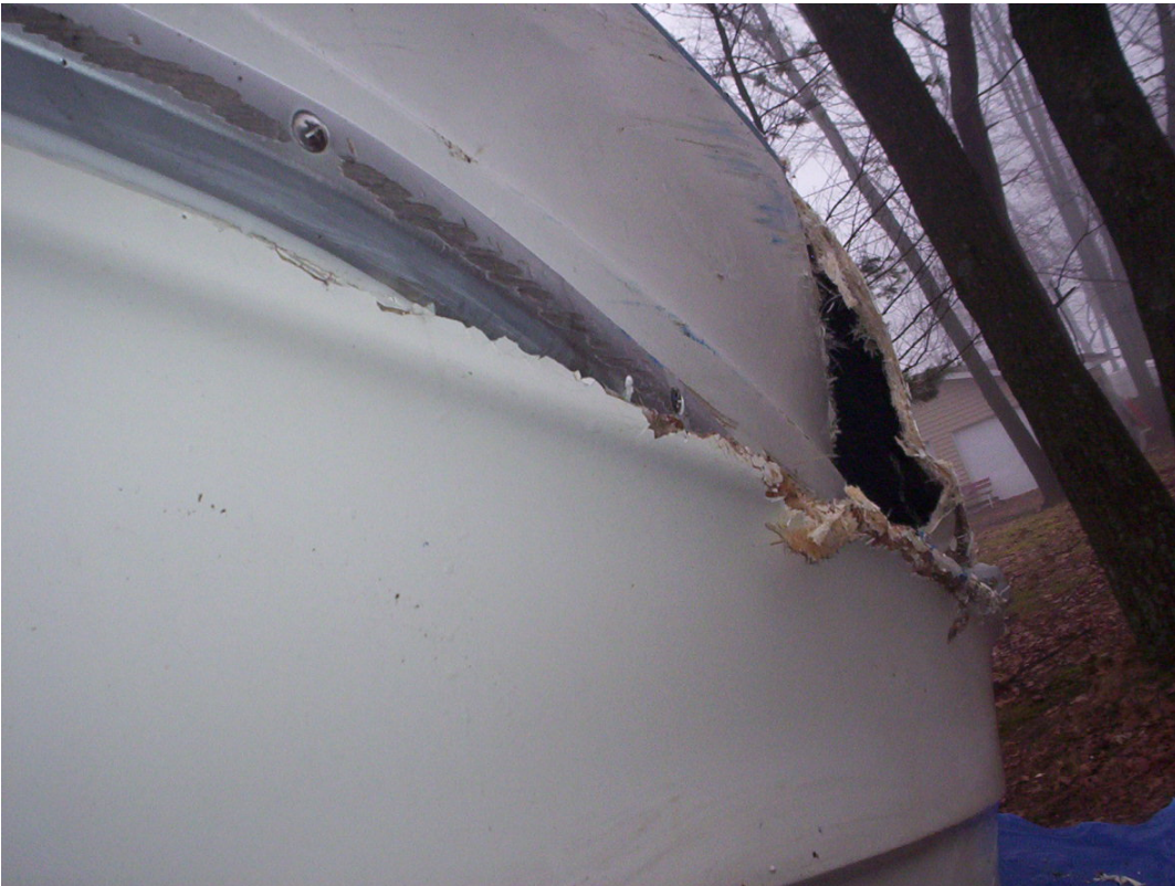
Deck and hull broken
