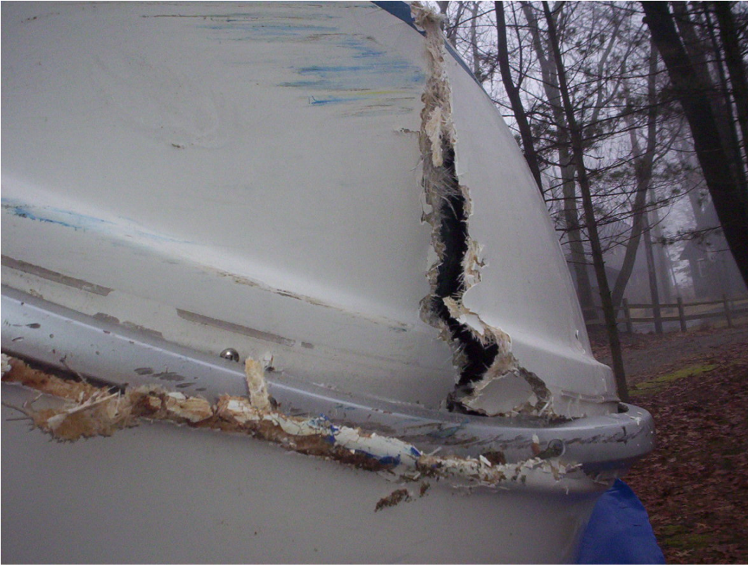
Cut shrinkwrap for estimate, several stress cracks extending out from repair.
